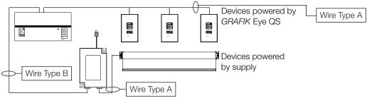
**Example:** Connecting to a *GRAFIK Eye* QS (**Note:** *GRAFIK* Eye QS powered from line voltage)
