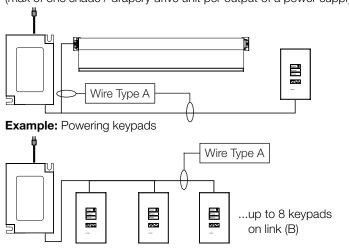
Example: Connecting to a GRAFIK Eye® QS (Note: GRAFIK Eye QS powered from line voltage)
